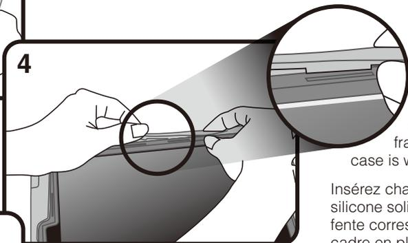
4 Insert each silicone tab tightly into its corresponding slot in the hard frame to ensure the case is water-resistant.
