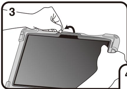
3 Insert the rest of the hard frame into the silicone cover.
