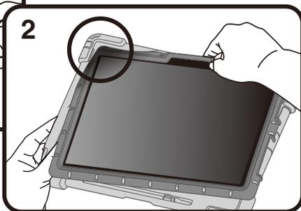
Insert the corner of the hard frame nearest the access port into the silicone cover.
